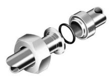
Ring Joint Type, RJT, unions are easily assembled and dismantled for cleaning purposes, this being a result of their having a Whitworth form thread. The RJT joint is not crevice free and may accumulate a deposit of the product being passed. However, present day cleaning systems are able to sanitise this area successfully without dismantling in the majority of applications. RJT unions may be operated at pressures up to 1.0 MPa.
