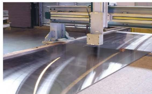
Laser equipment installed on this granite table checks MIC6 plates for flatness.
